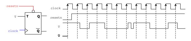
• Complete the timing diagram for the flip flop and the latch shown below: (7 pts)
