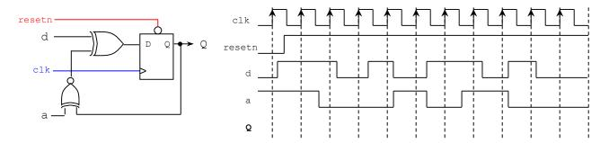
• Complete the timing diagram of the circuit shown below.  $Q = Q_3 Q_2 Q_1 Q_0$  (10 pts)
